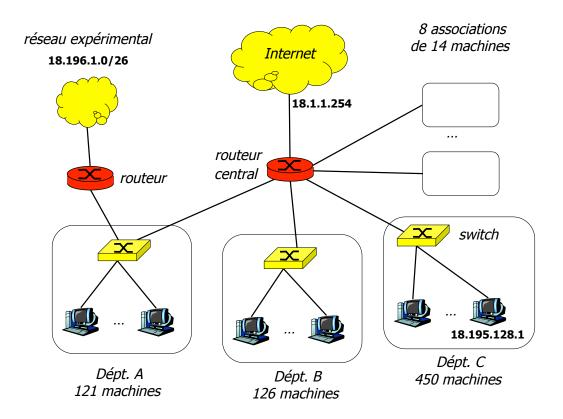
Figure 1: IP subnetworks of a company
