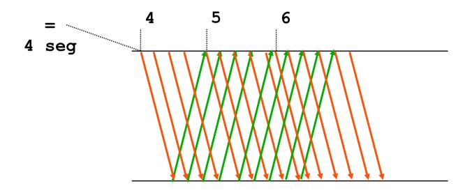
during one round trip + interval between packets: increase by 1 MSS (linear increase)
