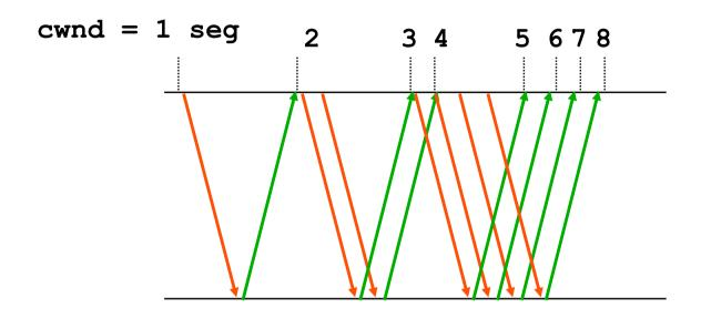
purpose of this phase: avoid bursts of data at the beggining or after a retransmission timeout
