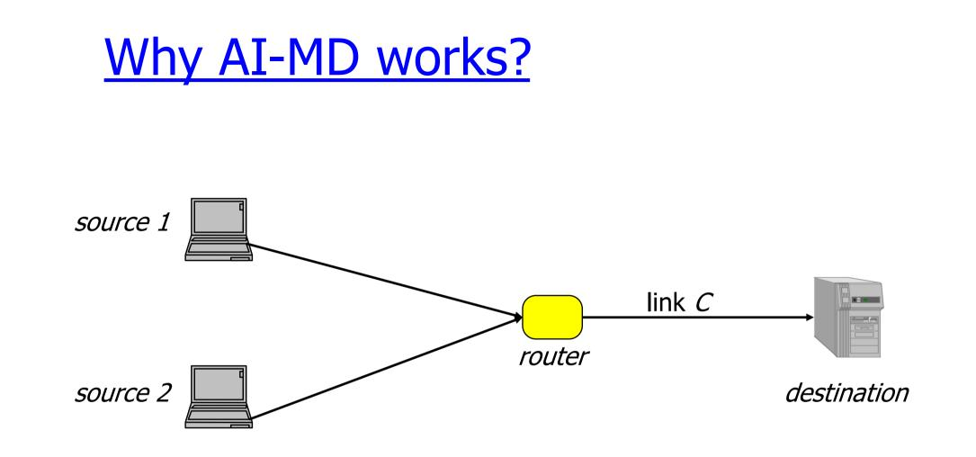
Simple scenario with two sources sharing a bottleneck link of capacity C
