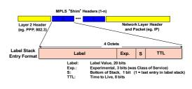
MPLS on PPP links and LANs uses shim header
